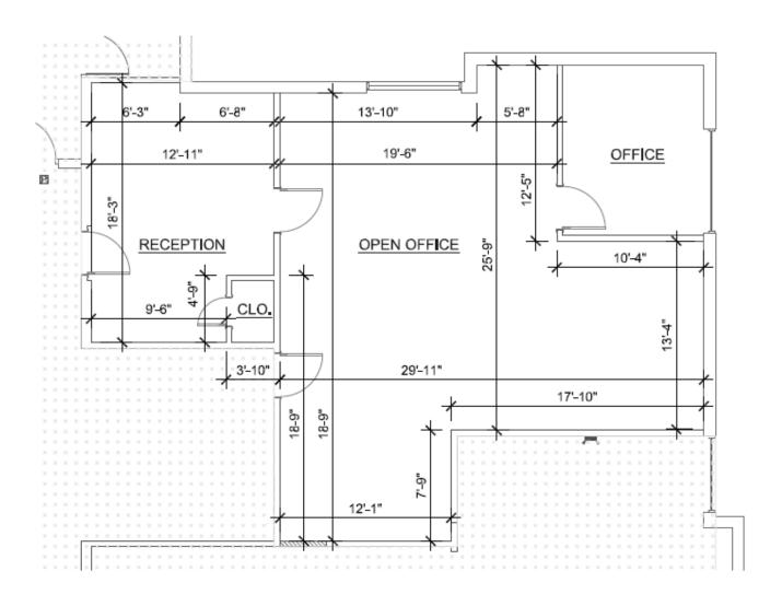
Floor Plan - Dimensions 1,092 RSF SCALE: 1/8" = 1'-0"
